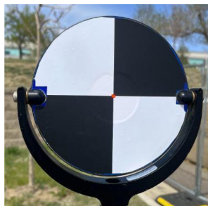
Figure 10: Visual confirmation of Laser Pointer on a target in the field
